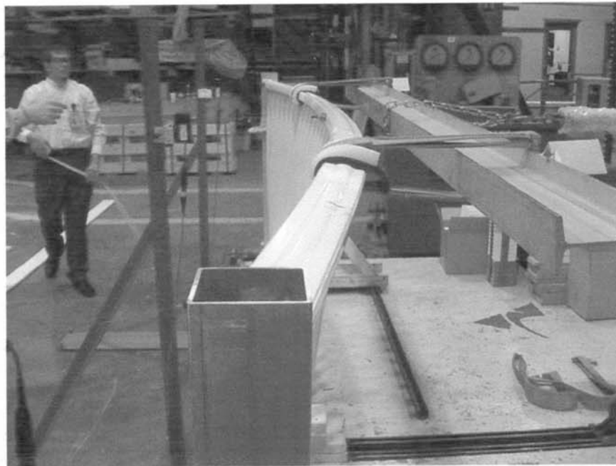
Photo No. 2 50 plf Top Rail Load Test
