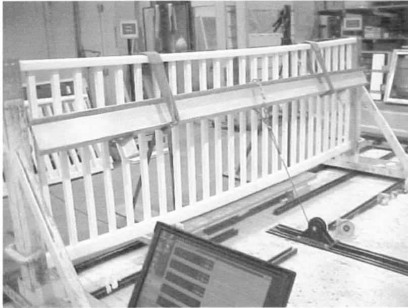
Photo No. 3 SBC Top Rail Load Test
