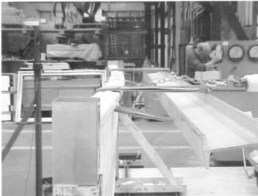
Photo No. 2 50 plf Top Rail Load Test
