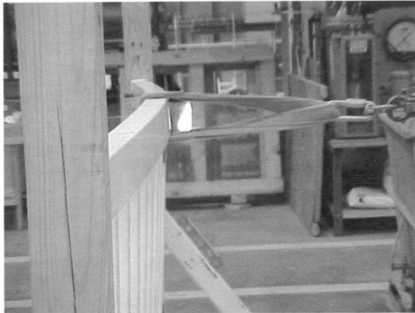
Photo No. 2 Top Rail Concentrated Load Test @ Mid
