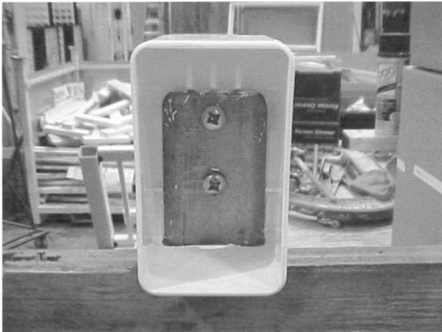
Photo No. 4 Bracket with Stainless Steel Plate
