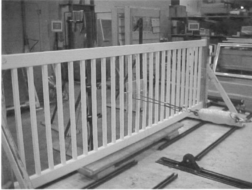
Photo No. 1 In-Fill Load Test
