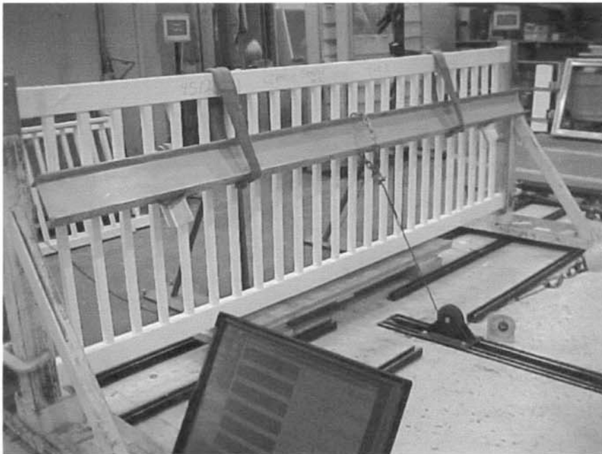
Photo No. 2 SBC Top Rail Load Test
