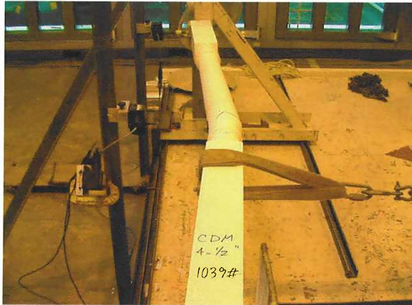
Photo No. 5 Lateral Load Test Typical Failure of Specimen (4-1/2" x 4-1/2" Porch Post)
