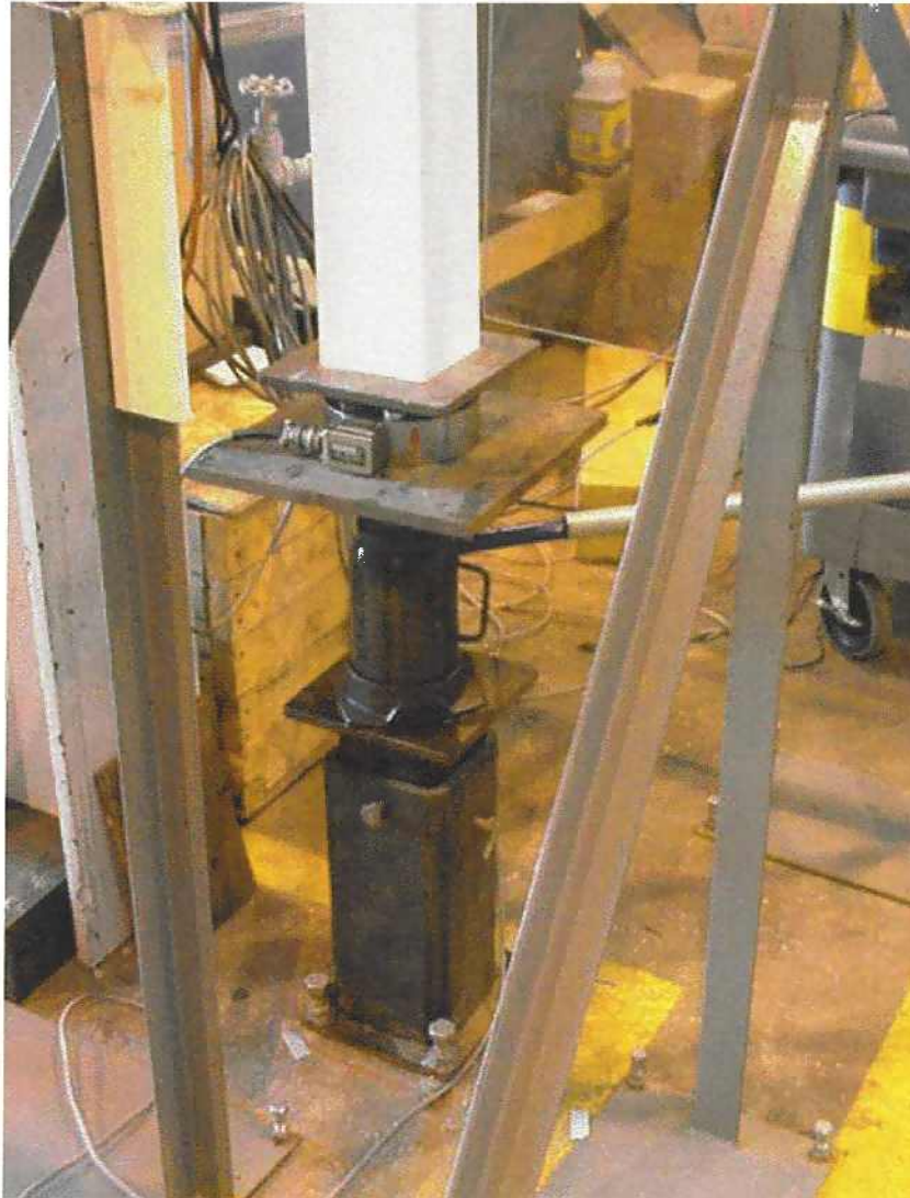
Photo No. 1 Column Base with Hydraulic Jack and Load Cell
