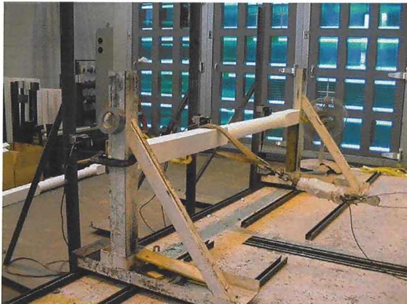
Photo No. 4 Lateral Load Test Setup
