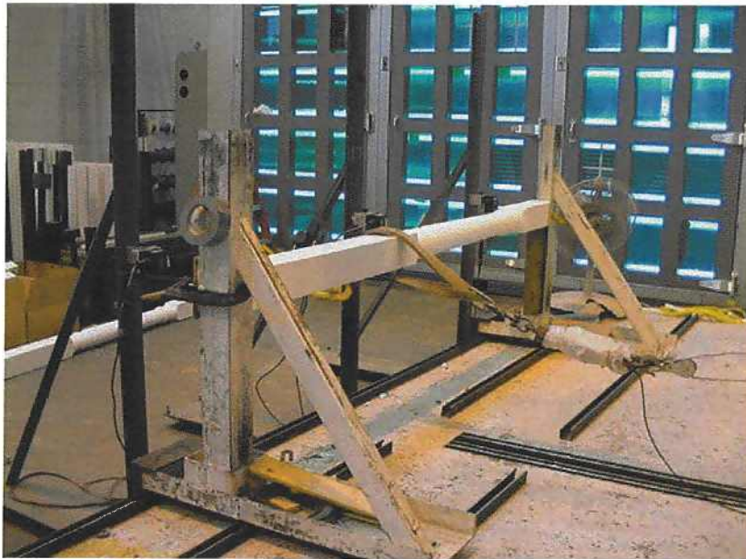
Photo No. 4 Lateral Load Test Setup
