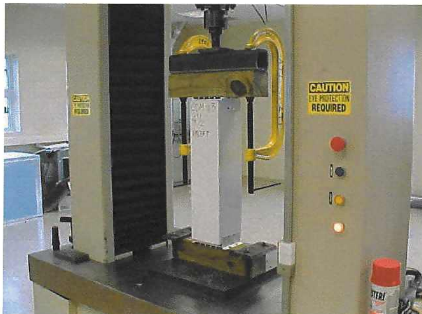
Photo No. 6 4-1/2" by 4-1/2" Porch Post Uplift Strength Test Setup
