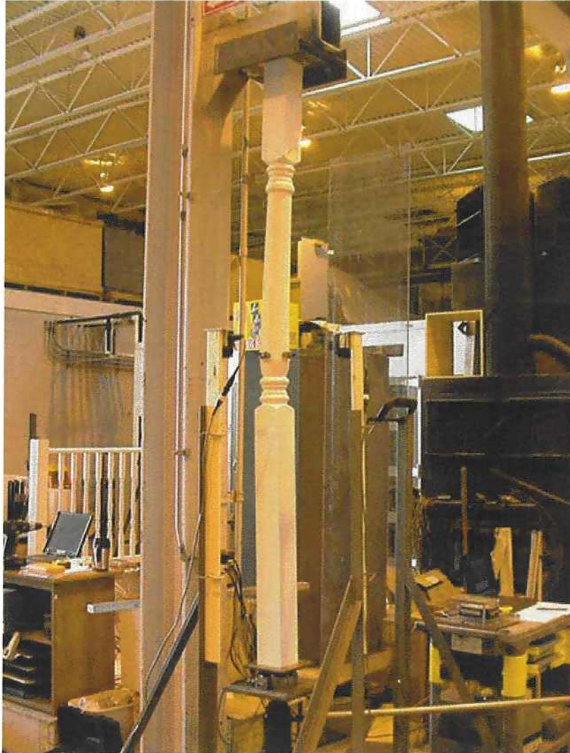
Photo No. 2 Axial Load Test Set-Up
