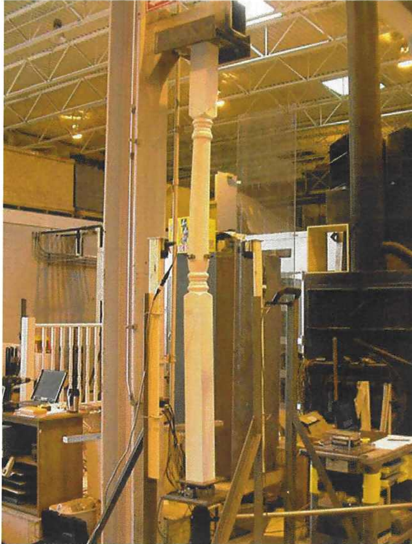
Photo No. 2 Axial Load Test Set-Up
