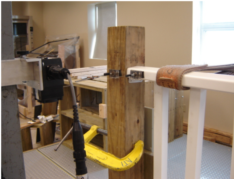
Photo No. 4 Concentrated Load on Top Rail Adjacent to a Post
