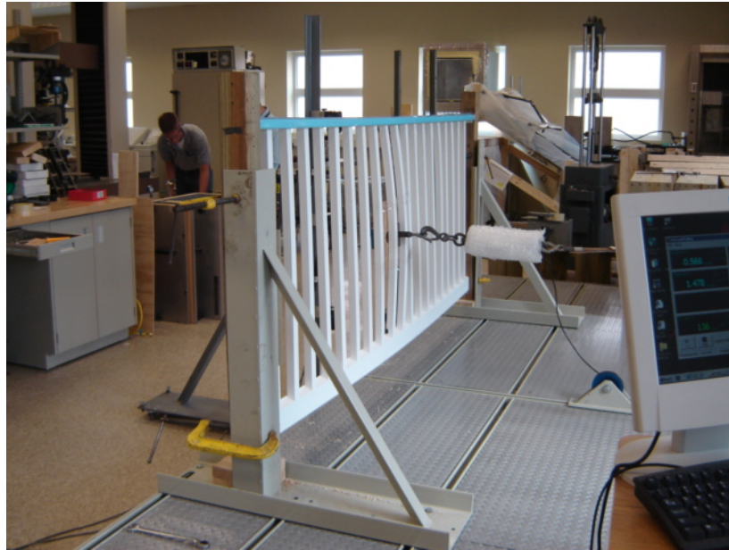
Photo No. 1 In-Fill Load at Center
