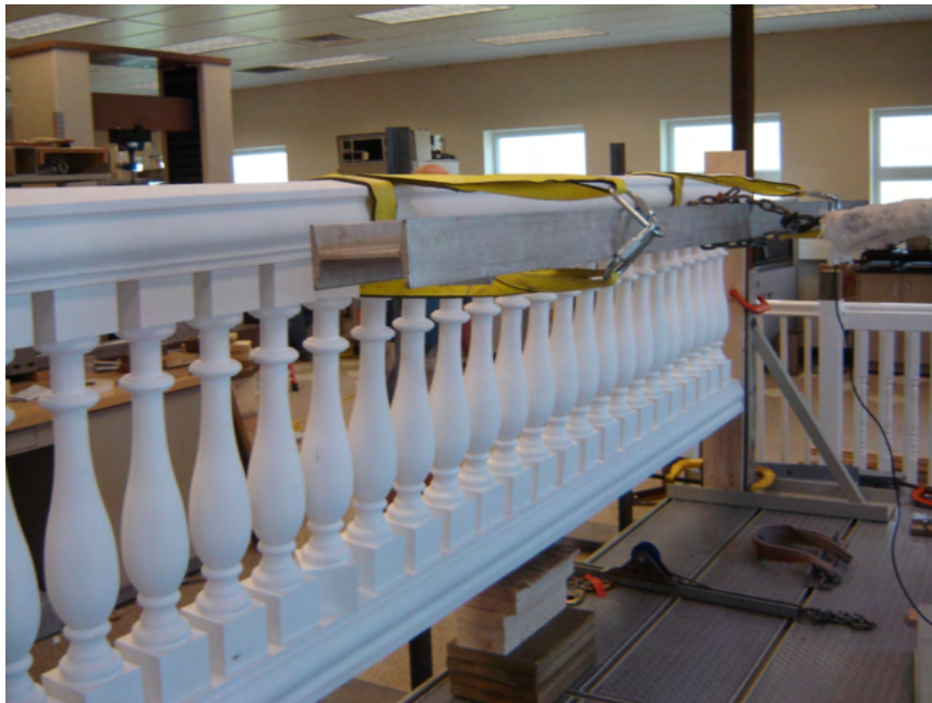
Photo No. 2 Top Rail Horizontal Uniform Load Test
