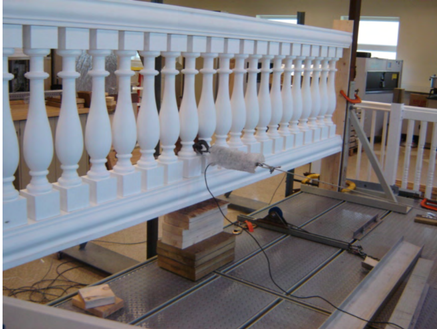
Photo No. 1 Bottom In-Fill Load Test
